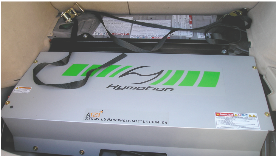
A123Systems' Hymotion Plug-in Conversion Module installed in the rear compartment of Toyota Prius, behind nickel metal hydride stock hybrid battery
